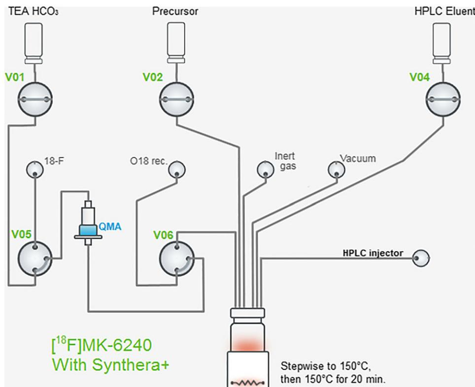
**FIGURE 1** Schematic diagram of the automatic synthesis module for the synthesis of  $[^{18}\text{F}]\text{MK-6240}$
