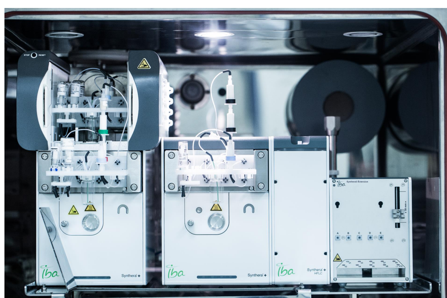
Synthera ® + platform: (from left to right) Synthera ® + synthesized with IFP loader, Synthera ® synthesizer, Synthera ® + HPLC & Synthera ® Extension
