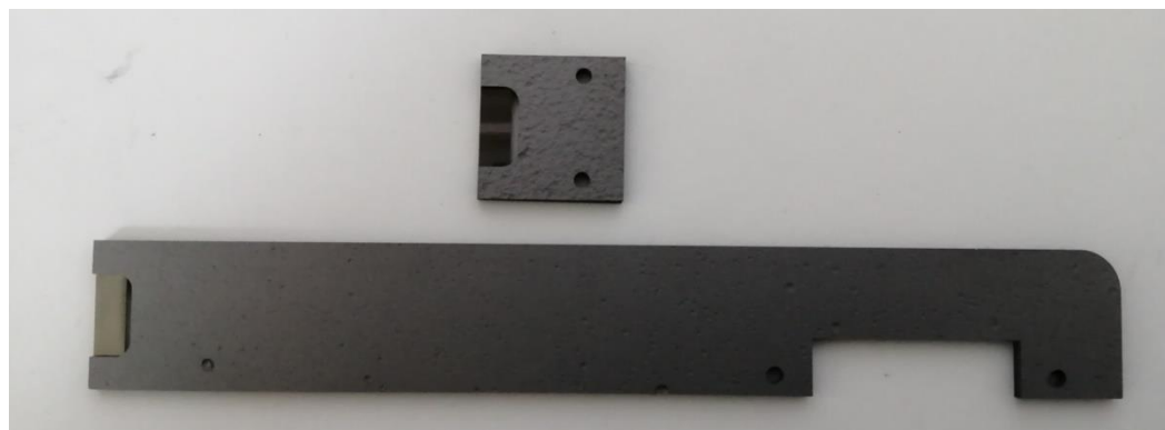
Figure 5. Stripper forks used to extract the proton beam with 13 (long fork) and 18 (short fork) MeV.
